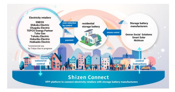
This service utilizes Shizen Connect's energy management system "Shizen Connect" to remotely control the charging and discharging of low-voltage energy equipment such as residential storage batteries, thereby creating a virtual power plant (VPP) that will generate reserves to help electricity retailers reduce their electricity procurement costs.
